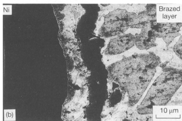
Figure 8 Scanning electron micrographs of brazed joints nickel-to-nickel with (a) alloy AR, (b) alloy AC, showing two distinct diffusion layers (a silver- and copper-rich layer close to the nickel base metal and, adjacent to this, a nickel- and silicon-rich layer).
